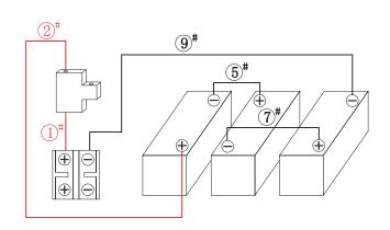
Note: Don't reverse battery polarities, or battery will be damaged
